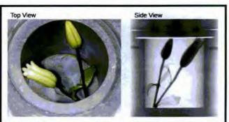
DARPA's Intense and Compact Neutron Sources (ICONS) program seeks to develop portable, next-generation imaging tools that combine the complementary benefits of X-ray and neutron radiography to enable highly detailed scanning in field settings. Neutron scanning provides the capability to see through many otherwise visually impenetrable objects; Asiatic lilies in a lead cask (left) are invisible to x-ray imaging but clearly visible in high resolution via neutron imaging (right).
