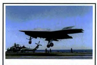
A Navy X-47B unmanned combat air vehicle demonstrator performs carrier operations.
